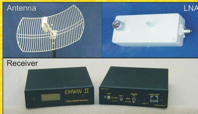
**Werner Labs** has developed a dual-mode receiver for the EMWIN-N format, that also works with the old one. Thus, purchasers can upgrade to the new receiver now, using it for the current satellites, and be ready for GOES 13 when it is activated.
